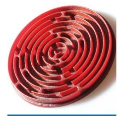
Photopolymer Jetting samples printed by Xaar 501 by DP Polar
