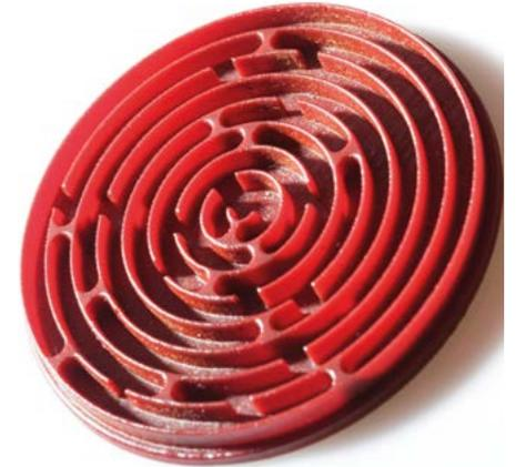
Photopolymer Jetting samples printed by Xaar 501 by DP Polar
